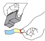
**6** Insert the inkjet cartridge into the cartridge bay with the label facing up and the gold contacts towards the front of the printer.
